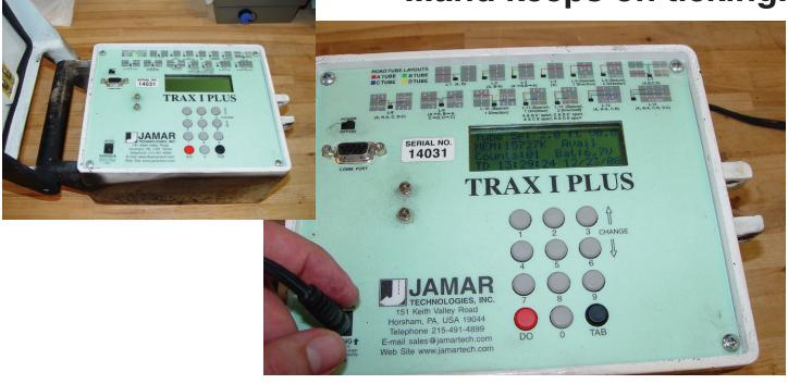
A customer recently sent in a TRAX I Plus that appeared to have been set on fire, badly burning the outside. We opened it up, hooked up power and the counter came right on, with a count still in memory. Even the date and time were still right.
